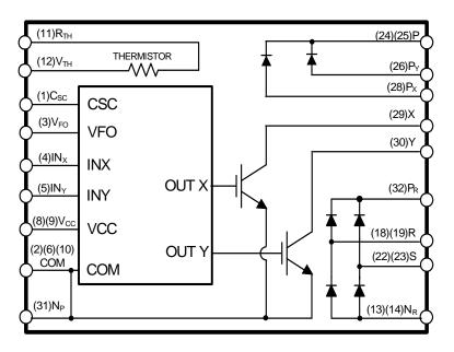
Figure 3. Internal Block Diagram
