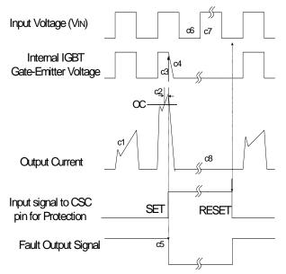
(with the external over current detection circuit)
