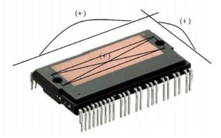
Figure 6. Flatness Measurement Position
