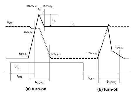
Figure 4. Switching Time Definition
