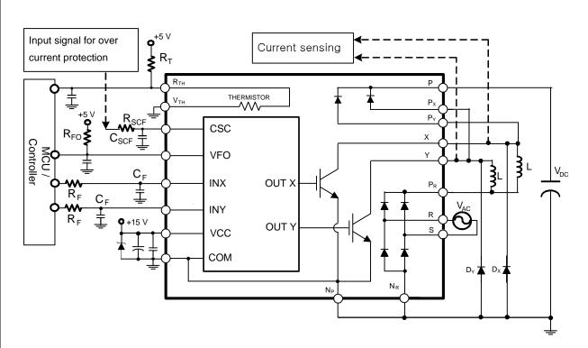
**Figure 9. Typical Application Circuit**
