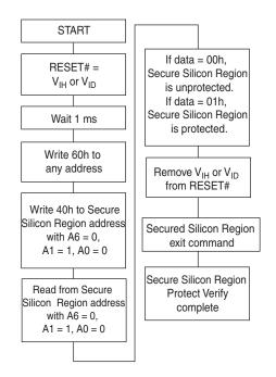
Figure 8.3 Secured Silicon Region Protect Verify
