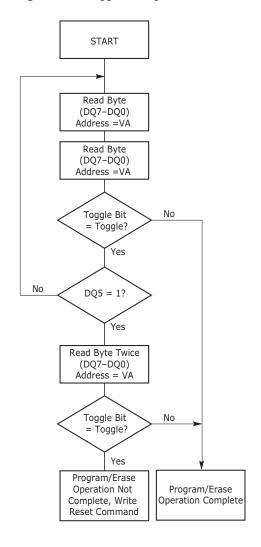
Figure 11.2 Toggle Bit Algorithm
