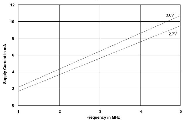
Figure 14.2 Typical  $I_{CC1}$  vs. Frequency
