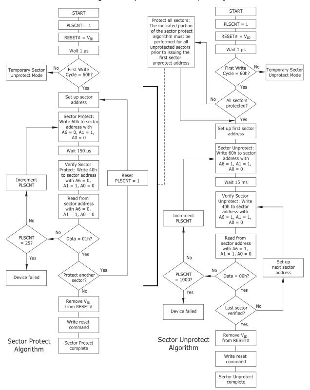
Figure 8.2 In-System Sector Protect/Unprotect Algorithms
