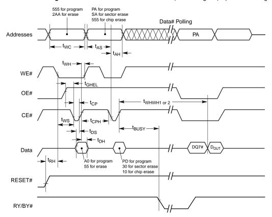
Figure 17.14 Alternate CE# Controlled Write (Erase/Program) Operation Timings
