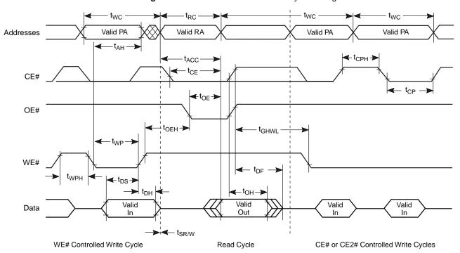
Figure 17.8 Back-to-back Read/Write Cycle Timings
