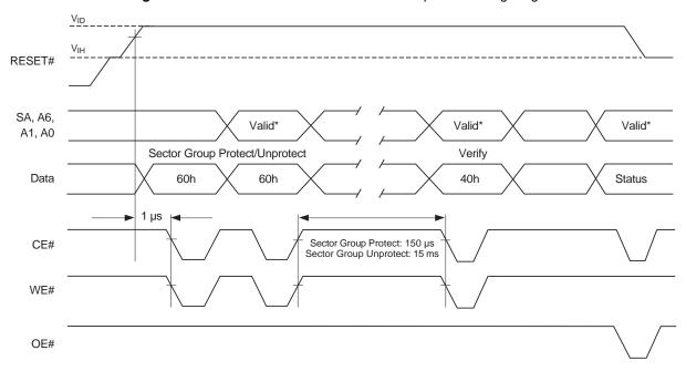
Figure 17.13 Sector/Sector Block Protect and Unprotect Timing Diagram
