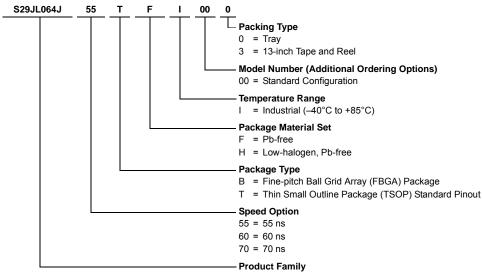
S29JL064J: 3.0 Volt-only, 64 Mbit (4 M x 16-bit/8 M x 8-bit) Simultaneous Read/Write Flash Memory Manufactured on 110 nm process technology
