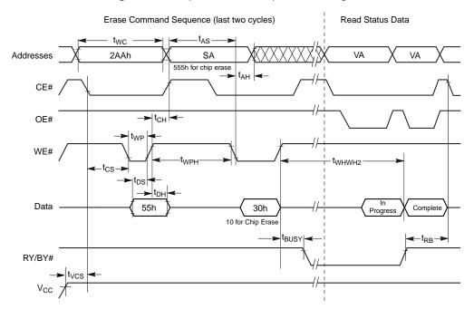
Figure 17.7 Chip/Sector Erase Operation Timings
