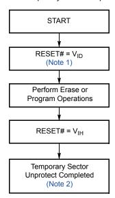
Figure 8.1 Temporary Sector Unprotect Operation
