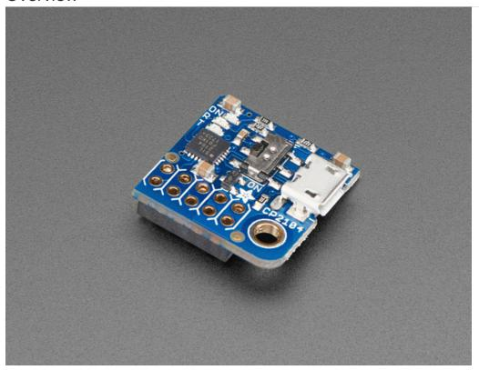
Here's another super handy add-on for your Raspberry Pi computer, perfect for 'head-less' setups! The PiUART adds a MicroUSB to serial connection so you can use any serial port software to connect to the Pi's console. It plugs in and is fast and easy to add whenever you need to connect to your Pi. Two LEDs connect to RX and TX on the serial converter chip so you get blinking whenever data is sent or received.
